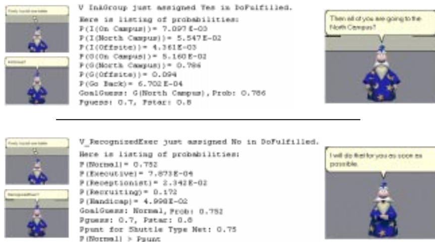
Figure 5. Upper sequence: Use of VOI to acquire visual information confirming the presence of a group, followed by update of probabilities for Level 1 goals and a decision to confirm a goal explicitly. Lower sequence: Progression to next level, use of VOI to detect if user is a recognized executive, update of probabilities of goals, and decision to forego interaction with the user about an atypical condition.
